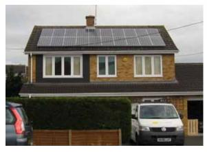
This large domestic solar PV system was installed in St Neots in November 2010. It has been designed to fill most of the available roof area and is rated at 3.6 kWp. This is ideal as it is a little lower than the 4 kWp threshold after which the financial rewards reduce slightly. The system is providing Mr and Mrs Welham with an income stream and savings on their electricity bills. This income stream is through the Governments 'Feed-in Tariff', a financial
